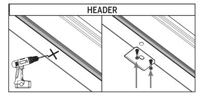
c. At the marked location on the header, drill a hole 3/8" in diameter and at least 1-3/8" deep. Install the header strike plate into the header, using two  $#8 \times 3"$  screws.
