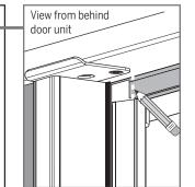
**a.** Close the inactive door. Make a mark at the location where the trim cap contacts the weatherstrip.
