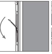
**b.** Engage the flip lever so the upper and lower bolt pins come in contact with the header and the sill. Mark these points of contact.
