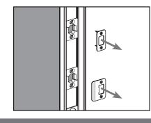
**a.** If installing new strike and deadbolt plates, remove the screws securing the old plates.
