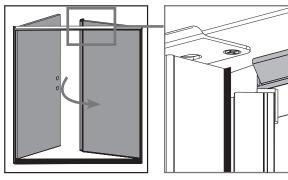
**c.** Close the inactive door panel. Ensure the weatherstrip forms a secure seal around the trim cap.
