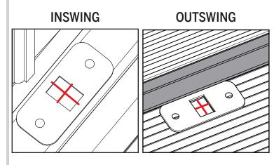
a. Using the marks you have made in Steps 7 and 8, line up the strike plate on the sill cap or deck.
