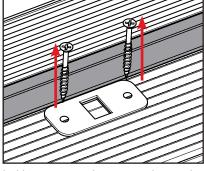
b. Unscrew and remove the strike plate.
